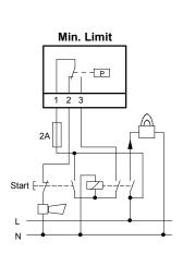
Pressure monitor as safety pressure limiter for falling pressure
