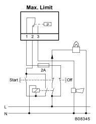
Pressure monitor as safety pressure limiter for rising pressure
