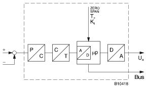
The filter time constant  $\tau$  of the transducer can be set to stabilise the sensor output signal in case of widely fluctuating pressure signals (see the technical data and fitting instructions).
