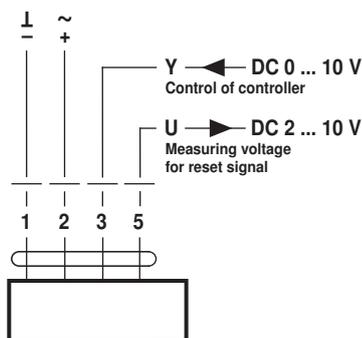
**Override control (frost protection circuit)**
