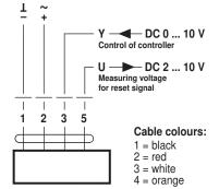
Override control (frost protection circuit)
