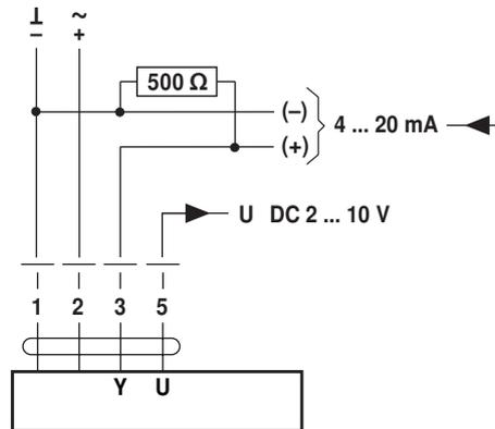
The 500 Ω resistor converts the 4 ... 20 mA current signal into a voltage signal DC 2 ... 10 V
